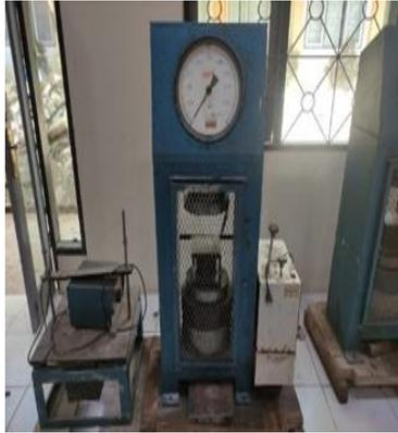
**Gambar 3. Compression Machine 2000 KN**
